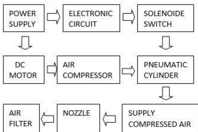
From this block diagram we get information about the component and how they are link up with each other. We take power supply from electric board for DC motor, Air compressor and electronic circuit by single wire. In electronic circuit there are three components.
